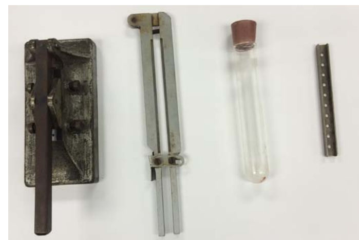
Fig 2: Components & Tools used for Test (l-r: nicking jig, bending and transfer tool, test tube, holding strip)
