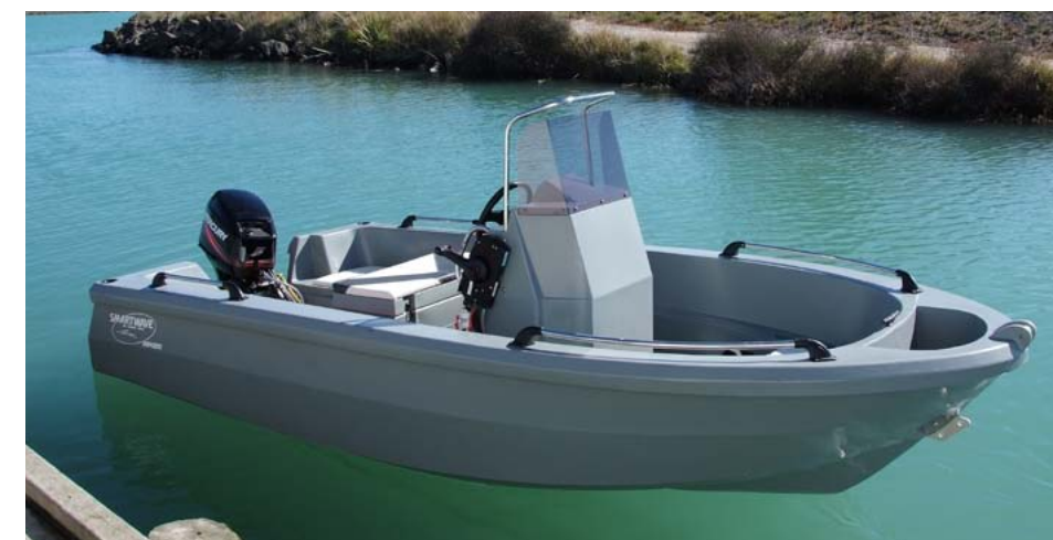
Smartwave 4200 boat, produced by David Hickmott & Advantage Plastics, Rangiora South Island NZ from Matrix Rotathene.
