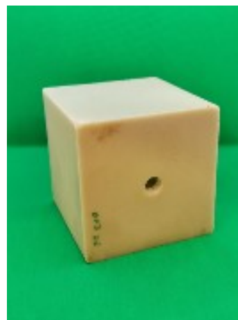
Photos of rotomolded parts from PE and FR series processed at 200, 250 and 300 °C.
