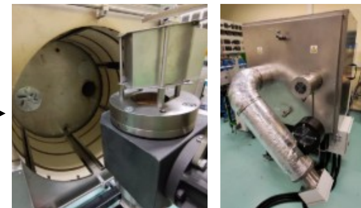
A prototype RotoLab-X rotational molding machine built for the project
